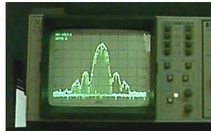
Wideband signal (transmitted SS signal)
