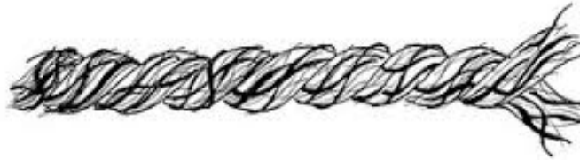
spun from blend of conductive and non-conductive fibers
