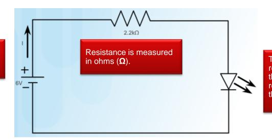
The triangular part represents a diode and the two arrows facing out represent the fact that this diode emits light.
