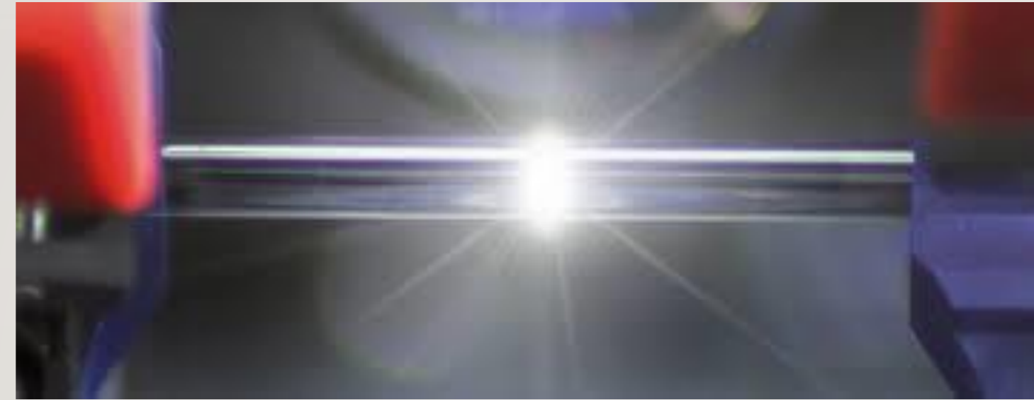
Gambar A. Fusion Splice Event
