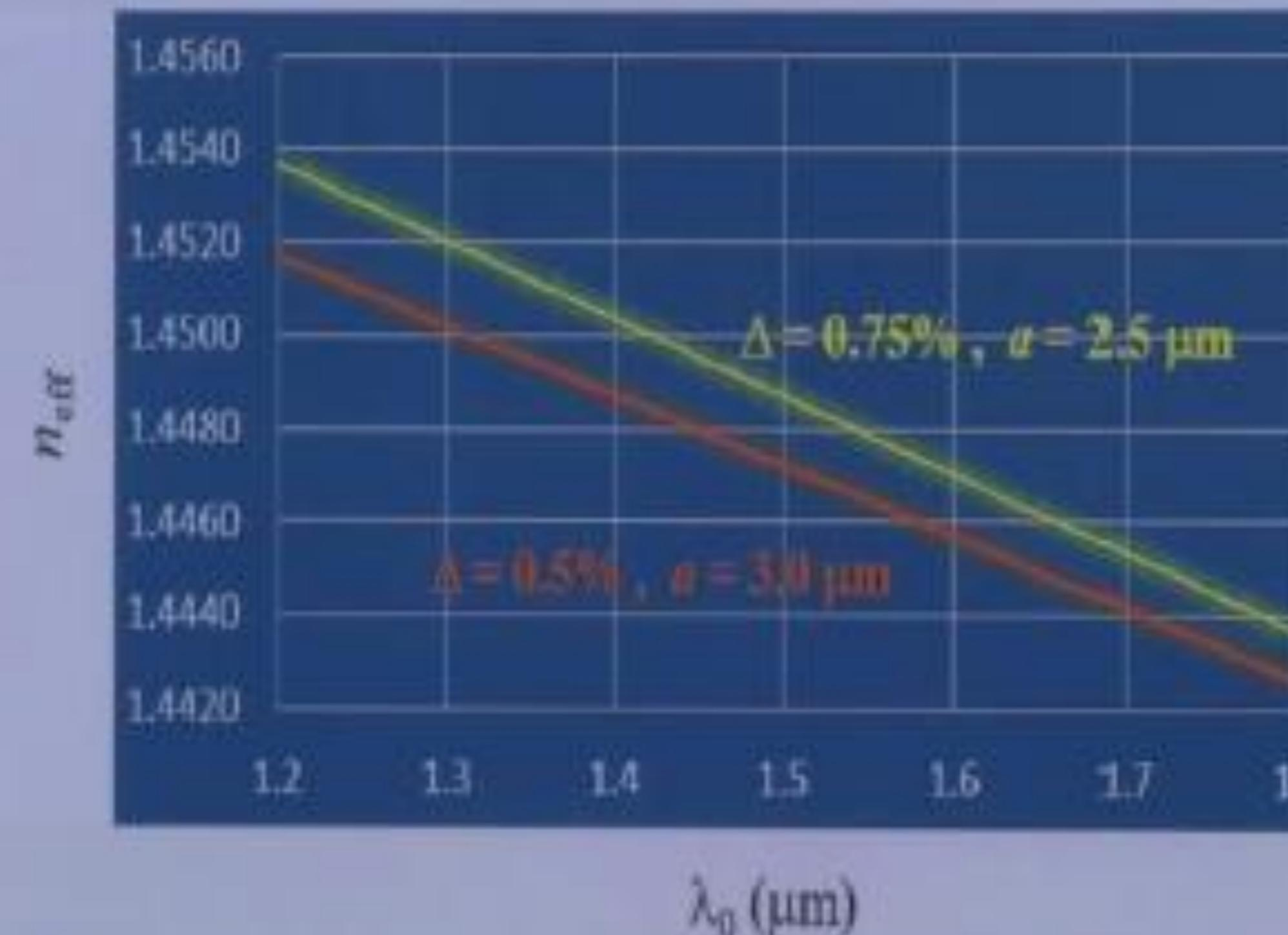
Slope of  $n_{eff}$  curve changes → waveguide dispersion is affected
